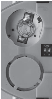
Left: Picture of the opened rear battery compartment of the RMT8-IR remote showing the exposed DIP Switch bank between the battery chambers.
