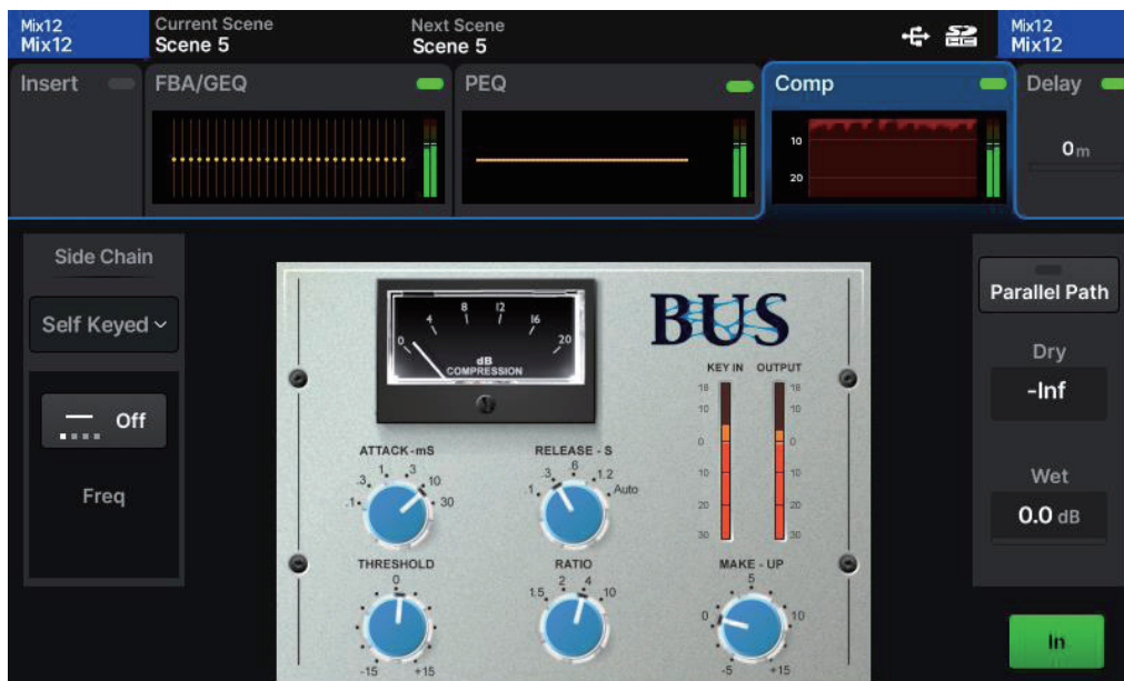
|| PROCESSING | DEEP Compressor (Mix Channel)
