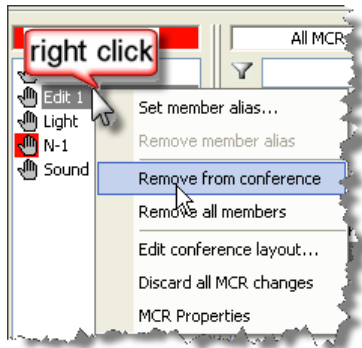
Figure 713: MCR handling - Remove a member with a right click in the conference
