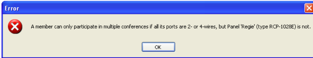
Figure 679: MCR – Error message when trying to use a panel in multiple conferences
