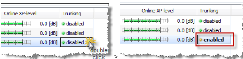
Figure 829: Trunking - IFB-Table - activate IFB
